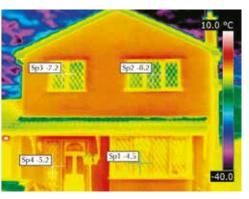
BEFORE and AFTER: The above thermal images clearly demonstrate the advantages of installing new energy efficient windows. The heat loss temperature of the living room window is  $1.3^{\circ}$ C before and  $-4.5^{\circ}$ C after the new windows were fitted - a significant reduction.
